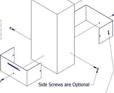
Slot Allows for Expansion/Contraction
